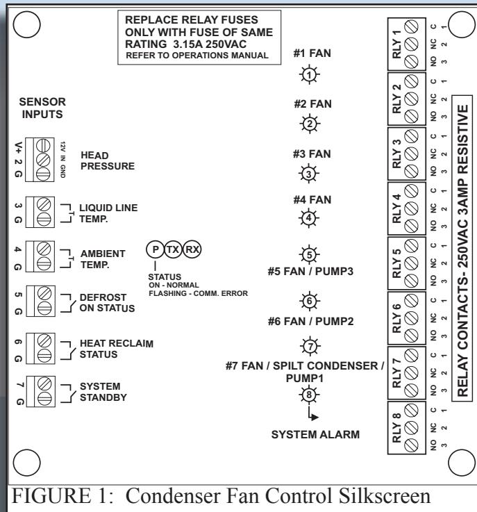
FIGURE 1: Condenser Fan Control Silkscreen
