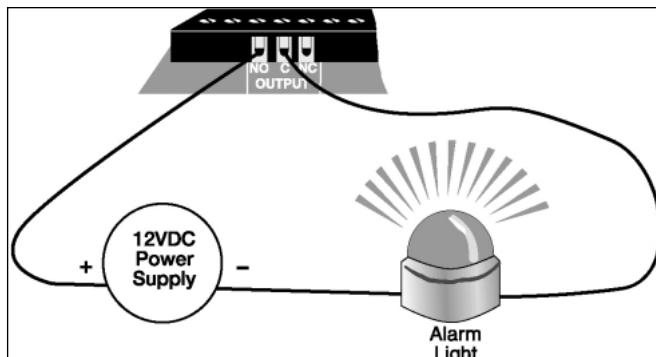
**NOTE:** For safety reasons it is highly recommended that the unit only be used to switch low voltage signals (30 volts or less). If you intend to control higher voltages you must install the unit in an NEC approved electrical panel or enclosure and have wiring performed by a qualified electrician.
